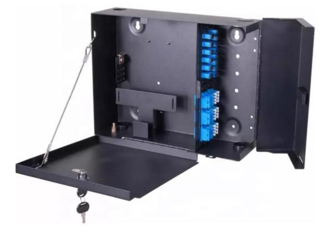
Distribution box series are applicable in FTTH project and suitable for building's outer walls application; They can distribute cables after installing splitters and also can draw out room fiber optic cables by direct or cross-connections. They are with the function of mechanical splice, fusion splice, light splitting, wiring distributions etc.
