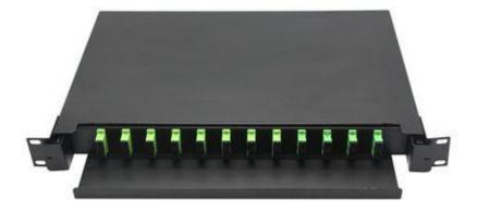
19" Rack mounted Fiber Duplex Patch Panel. Fixed type splice tray for Pigtail splicing. Available in LC, SC connector adapters. Lockable front door. Patch panel is made up of cold rolled steel sheet.
