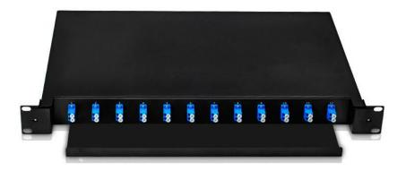
19" Rack mounted Fiber Duplex Patch Panel. Fixed type splice tray for Pigtail splicing. Available in LC, SC connector adapters. Lockable front door. Patch panel is made up of cold rolled steel sheet.
