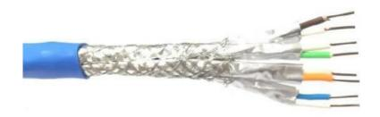
Cat8 S/FTP cable constructed with 4-pair, 22 AWG conductor. Available in 305 Mtr per Roll.
