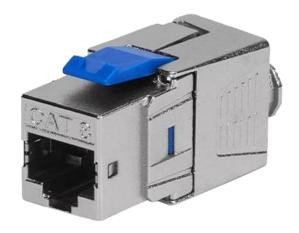
Network module is a kind of high speed, high performance and flame retardant data module. As a kind of network accessory, it plays a role of intermediate connector, and we can also think it as a data transit station. The network module is mainly working with patch panel, faceplate, and distribution box.
