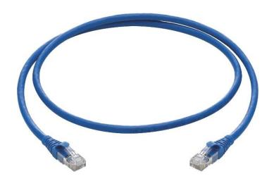
Cat8 S/FTP patch cable features 26AWG unshielded twisted pair stranded copper cable with a high performance modular plug at each end. Snagless design protects the locking clips on the RJ45 connectors from being damaged or snapped off during installation.
