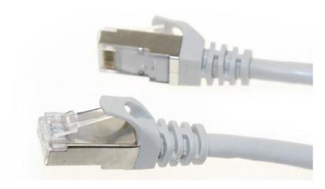
Cat6 S/FTP patch cable features 23AWG unshielded twisted pair stranded copper cable with a high performance modular plug at each end. Snagless design protects the locking clips on the RJ45 connectors from being damaged or snapped off during installation.
