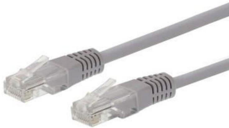
Cat6A UTP patch cable features 23AWG unshielded twisted pair stranded copper cable with a high performance modular plug at each end. Snagless design protects the locking clips on the RJ45 connectors from being damaged or snapped off during installation.
