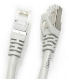
Cat6A S/FTP patch cable features 23AWG unshielded twisted pair stranded copper cable with a high performance modular plug at each end. Snagless design protects the locking clips on the RJ45 connectors from being damaged or snapped off during installation.
